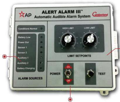
These Limit set points consist of high and low limit. When it detects the temperature reaches the high/low, it will trigger the alarm. When this happens, main controller might be faulty.
